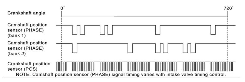
Inspect cam encoder positions as shown above by removing sensors.
