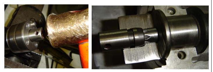
Final inspect the assembly. Remove the O-ring dampener from the female coupling on the new
