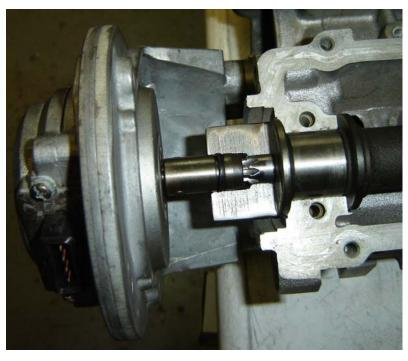
wearing at an alarming rate. A technical service bulletin was issued when it was discovered that the cause was a slight eccentricity in the alignment of the CAS to the camshaft, caused by a machining error of the CAS mounting bracket to cylinder head aligning dowel holes.
