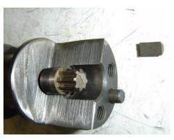
9. Thread an M6 bolt into the hole until it contacts the cam behind the CAS pin; continue tightening the bolt until the CAS pin is pulled out of the hole.
