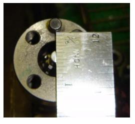
12. Using the female coupling you removed from the old CAS and a hammer, tap the CAS drive pin slightly into the cam and check that it's rotational position is correct before seating the CAS pin. If the alignment is good, continue to seat the CAS pin until the female coupling bottoms in the shoulder hole, as shown (the hammer feedback will feel distinctly more solid).
