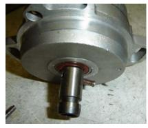
11. To install the new CAS drive pin, support the cam so that damage to lobes and bearing journals is not possible. When installing the CAS drive pin into the camshaft, insure that it is exactly aligned as shown, with the half round extension positioned on the left (9:00 o'clock if the cam dowel is at 12 o'clock) and the straight edge aligning with the middle of the cam dowel pin.
