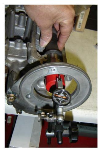
Note: If you have a new CAS mount, test fit it to determine if any eccentricity is in your mount or the head. If your original error is repeated with the new mount, the error is with the head, if it is concentric with the new mount, you are done, use the new mount! If not, continue.
