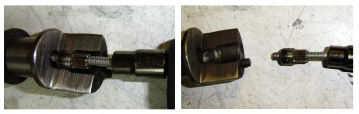
10. If you are installing a new CAS unit, remove the female coupling from the end of your old CAS unit by using a drift punch to remove the retaining pin. This will make the perfect tool for pressing the new CAS drive pin into the camshaft. If not you will need to make a sleeve suitable for pressing the CAS drive pin into place; it must sit snug on the shoulder below the spline section.
