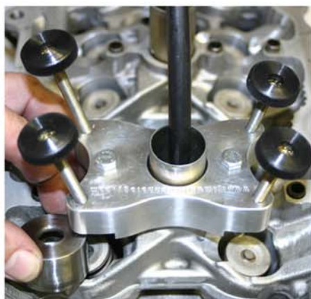
Install the supplied bucket over the valve. Make sure the bucket moves smoothly and is not binding.
