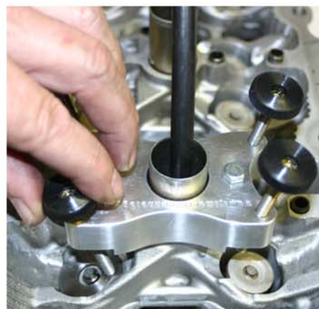
Lower the screw until it contacts the bucket, and rotate it 5 rotations. Stop if any binding is felt and investigate!
