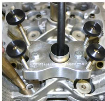
Tap the bucket with a brass or plastic punch to unseat the spring retainer locks before compressing the spring.
