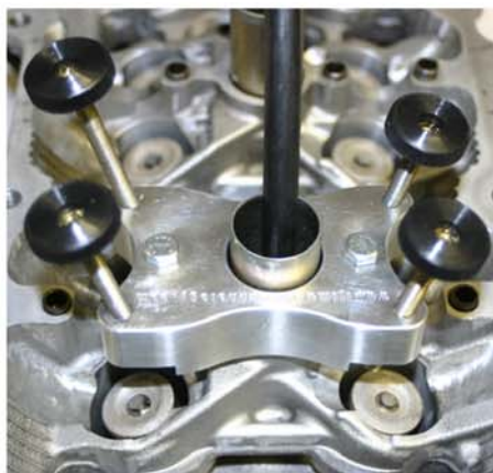
Bolt the tool to the head using the 2 inboard cam bearing cap bolt holes
