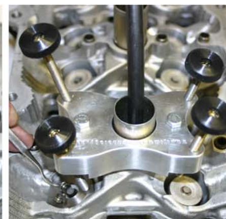
On reinstall, compress the bucket and drop the retainer locks onto the bucket and move them into place.
