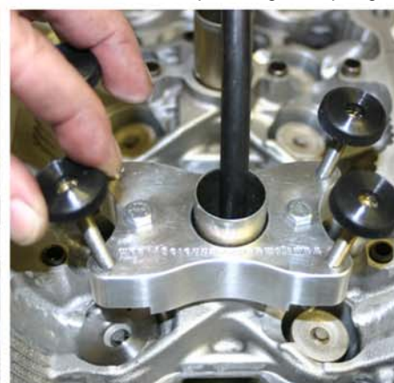
Back off the screw fully into the tool.
