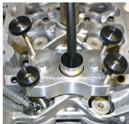
Using a magnet or a dental pick, remove the retainer locks
