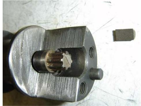
9. Thread an M6 bolt into the hole until it contacts the cam behind the CAS pin; continue tightening the bolt until the CAS pin is pulled out of the hole.
