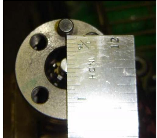
12. Using the female coupling you removed from the old CAS and a hammer, tap the CAS drive pin slightly into the cam and check that it's rotational position is correct before seating the CAS pin. If the alignment is good, continue to seat the CAS pin until the female coupling bottoms in the shoulder hole, as shown (the hammer feedback will feel distinctly more solid).
