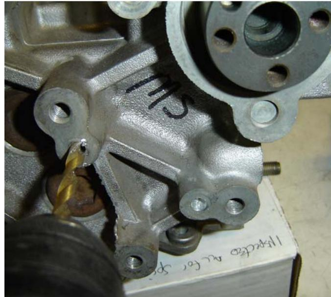
4. The dowel pins should be a slip fit into the CAS mount holes (they should go in and out of the holes by hand). Clean the dowel pins and remove any burrs from the holes until the dowels can be slipped in and out of the holes by hand. This will allow the dowels to stay with the head during any future disassembly.
