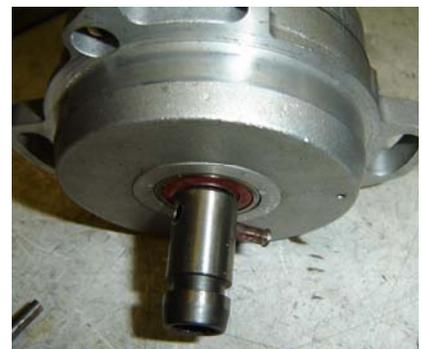
11. To install the new CAS drive pin, support the cam so that damage to lobes and bearing journals is not possible. When installing the CAS drive pin into the camshaft, insure that it is exactly aligned as shown, with the half round extension positioned on the left (9:00 o'clock if the cam dowel is at 12 o'clock) and the straight edge aligning with the middle of the cam dowel pin.
