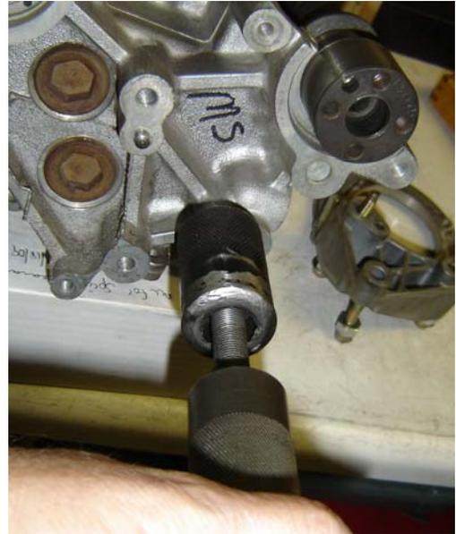
3. Drill out the dowel holes in the head with a  $\frac{1}{4}$ " drill if the eccentricity is less than  $.012$ " TIR, else use a drill that is large enough that the aluminum mount can be aligned.
