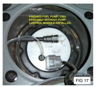
NOTE: This picture does not show a fuel pump control module signal tee'd into the 1/8" nylon tube. A Tee will be spliced in later if a fuel pump control module is used.
