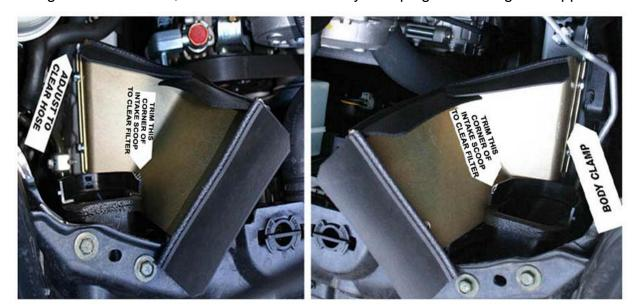
clamps and bolts to the edge of the car body frame rail as shown. It is extremely important the metal heat shields are positioned for and aft so they are not touching any existing hoses or hardware that may be damaged by the shields cutting into them.
