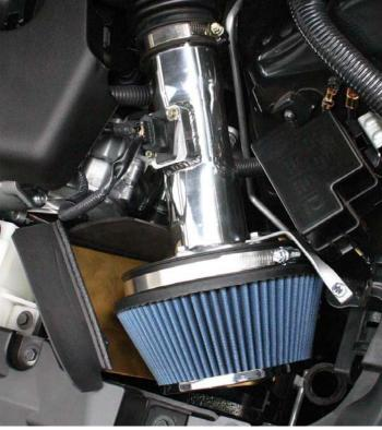
6. Determine which Pop-Charger air tube and filter assembly will go on the left side and right side. They are both identical except that one of the four-filter assembly bolts, closest to the fender has been left out for the mounting bracket. Install the filter / air tube
