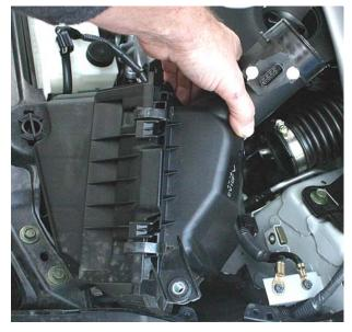
2. Transfer the MAF sensor from the original boxes to the new Pop-Charger air tubes; the bolt patterns are offset so you cannot put the sensors in wrong. This is a good time to remove the filter elements from each assembly and make sure there is no packing material or other foreign material inside the assembly before installation.
