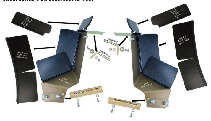
4. Using a 10mm wrench, install the heat shields by clamping them to the body frame rail using the supplied lower clamps as shown. It is extremely important the metal heat shields are positioned for and aft so they are not touching any existing hoses or hardware that may be damaged by the shields cutting into them. Trim the corners of the existing plastic air inlets as shown to clear the new filters.
