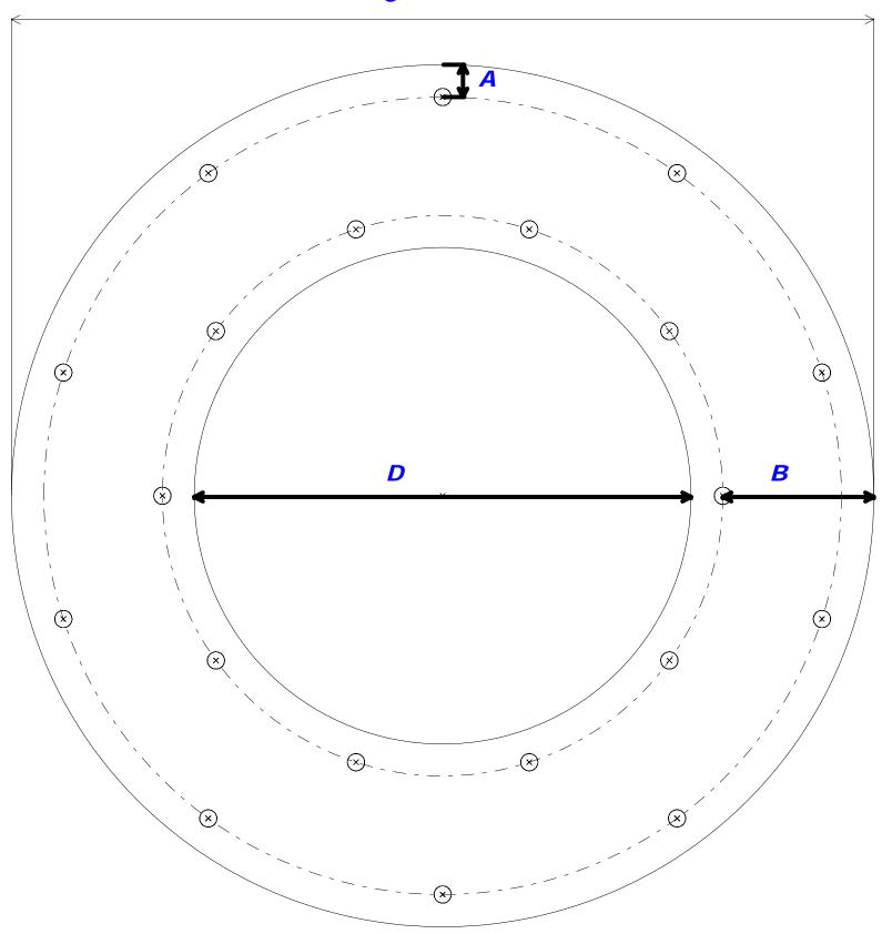
HEAT SHIELD DIMENSIONS NEEDED: NUMBER OF HOLES IN EACH BOLT CIRCLE.
