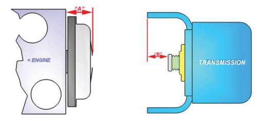
Measurement "A": On the engine side with the flywheel and clutch installed: measure the distance from the engine / bellhousing mating surface to the clutch release fingers.
