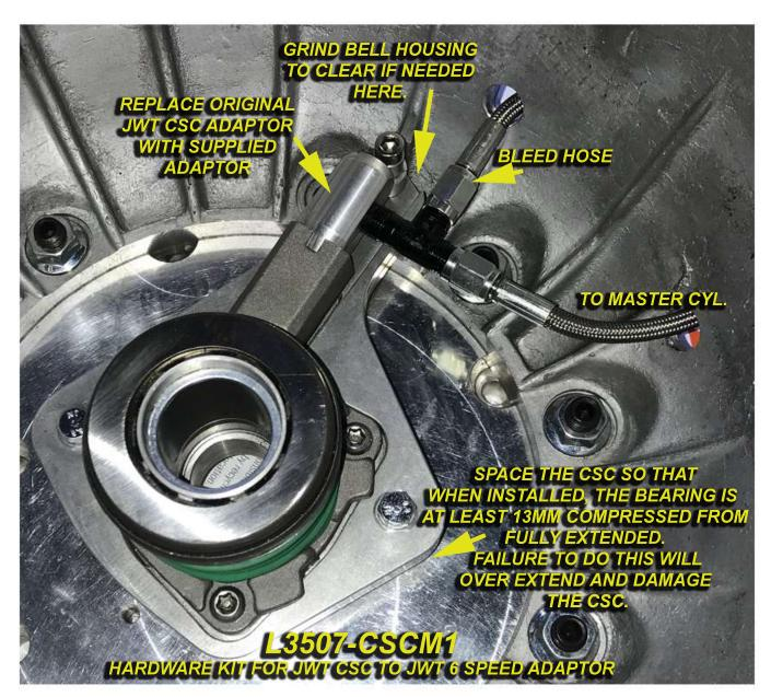
Due to the many combinations of clutches, flywheels, & bellhousings, this hardware is a starter kit that includes nominal CSC spacers that may need modification based on your specific installation. You must space the CSC so that it is compressed by 13mm from fully extended when installed to avoid over extending and damaging the CSC during operation. Most typical clutches will fully release with 7.5 to 8 mm of CSC travel and will fully release properly by this 13mm setting with a safety margin.
