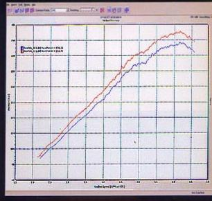
The Pop Charger bumped up peak horsepower by 14.4, with 12-16 horsepower gains realized between 4,500 and 5,200 RPM. Had we baselined the Z33 with a fresh factory filter, we estimate that the peak gains would probably be around 6 horsepower.
