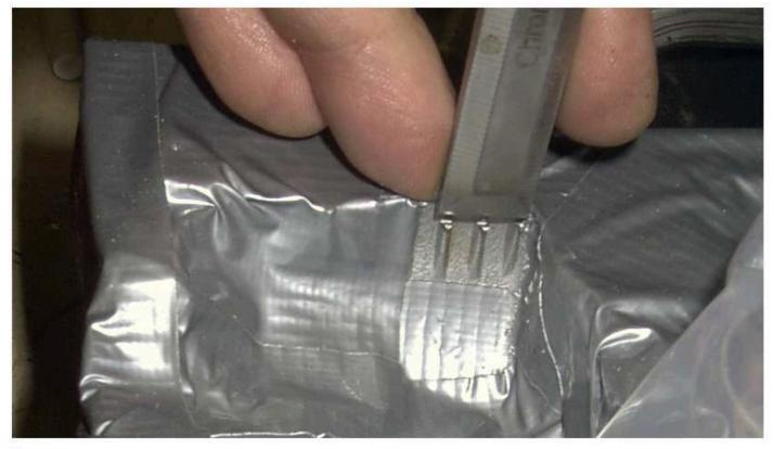
Completely seal off the head except the area to be clearanced using duct tape and plastic sheet (if the head is assembled). A sharp chisel can be used to cut away the 3 ribs that interfere with the front intake lobe. Remove all aluminum chips and tape, and check the cams for clearance before final assembly.
