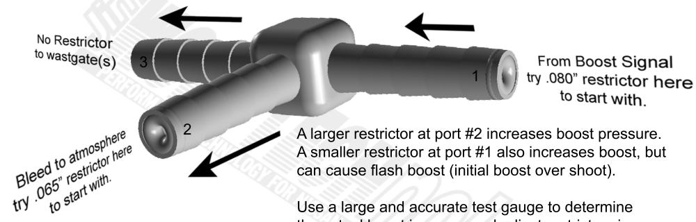
Use a large and accurate test gauge to determine the actual boost increase and adjust restrictor sizes as needed. Caution: Excessive boost, inadequate octane or tuning will cause knock (detonation) which can destroy your engine!
