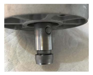
G. Install the CAS oil seal flat side out using an appropriate diameter tool. Press in until the it is flush with the CAS Base Housing surface. Apply a small amount of grease to the lip of the seal and the female splines that will engage the CAS Drive Pin and install the CAS and it's 3 locking bolts and washers.
