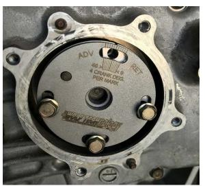
operation and must be locked in a position to avoid this. If the later is NOT the case, typically starting in the middle of the phaser travel (20degrees) is a good starting position. Torque the 4 lock plate bolt to 10 ft-lbs. using Loctite.
