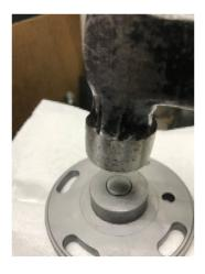
D. Install the Cam Lock Plate in the intended position the same as bank #1. (see #6 main instructions)
