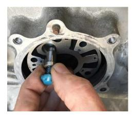
4. Measure the diameter of the home lock pin and choose the supplied Drive Pin Bushing that is the same diameter. Install the correct size Drive Pin Bushings and Drive Pins on both sides.
