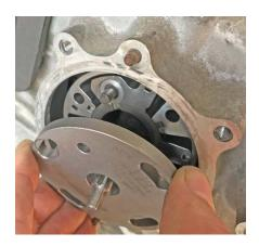
6. Adjust the Phase lock plates to set the intake cams to the degrees that you want them positioned. NOTE: Typically, this will be determined by dyno testing for the optimum results for the type of performance activity the engine is intended. The position may also be determined based on a cam, piston valve relief, valve diameter combination that would interfere at some intake cam position during normal phaser
