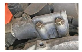
8. Install the supplied sprocket cover plates using silicone sealant. If you are using the optional VG30DE CAS Adaptor, only install the bank 1 cover, as the Adaptor will be installed on the bank 2 side.
