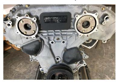
2. Remove the 4 bolts holding the phaser sprocket covers and discard the phaser sprocket covers. Be careful not to let the Home lock pin & spring fall as you remove the covers.
