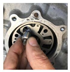
5. Install the supplied Phase Lock Plates, engaging them to the Drive Pins and loosely install the original bolts. NOTE: If you are using the optional VG30DE CAS Adaptor, see the addendum instructions at this point.
